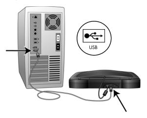
If the plug does not attach easily, make sure that you are plugging it in correctly. Do not force the plug into either connection.
